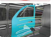
Coverage Map - View applied paint vs. target dry film thickness to see where paint is too thin, too thick, or within coating specifications.
