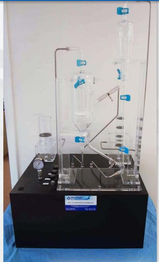
**Fluid Catalytic Cracking Working Demonstrator (132-FCCU)**
