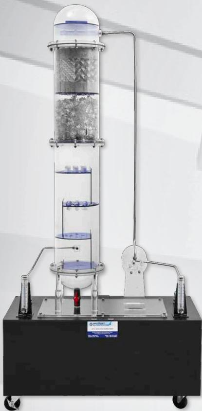
**Distillation Tower Working Demonstrator w/ Reboiler (132-DTT5)**
