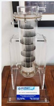
**Vertical Thermosyphon Reboiler Model (115-VTR)**
