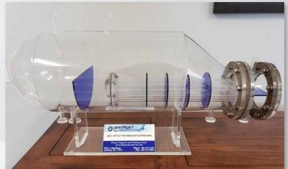
**Kettle Type Reboiler Floating Head Model (115-KRFH)**
